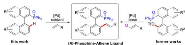
Scheme 1. Different Pathways for Synthesis of Phosphine–Alkene Ligand
